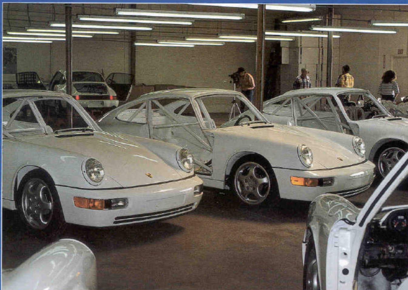
After Andial shipped the cars out for installation of the roll cage, they began installing a new electrical system, a different suspension, an on-board fire system and related safety equipment
