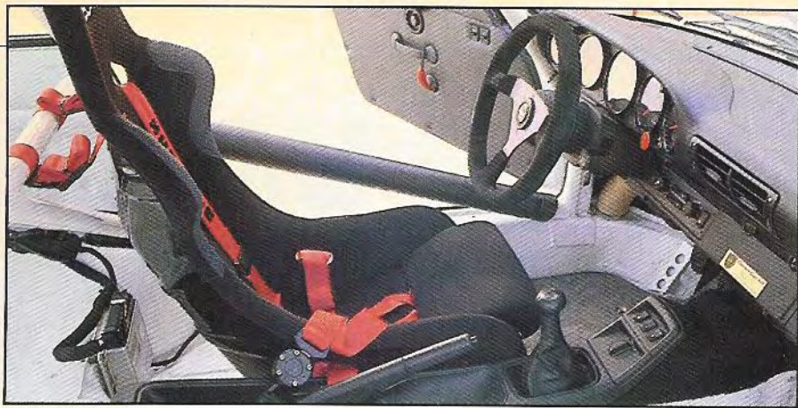
Altered interior among 110 hours of modifications to turn street car into Carrera Cup racer
