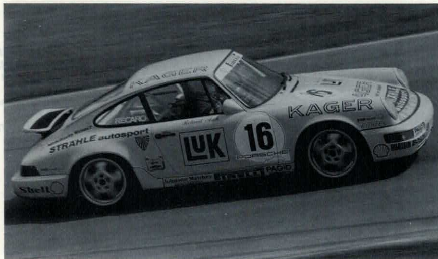
The for-racing-only 911 Carrera Cup car weighs in at about 2500 pounds and produces 271 horsepower from its competition-tuned 3.6-liter six cylinder.
